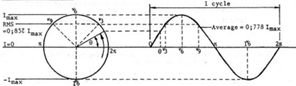
Current cannot rise for ever. To exploit inductance (and many other things) alternating current is used. Generated by rotating machinery the magnitude rises and falls like a spot on a steadily turning wheel. It is called sinusoidal for it is always proportional to the sine of the angle turned to at each moment.
